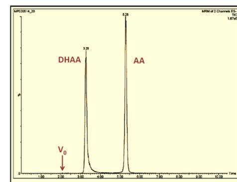
Figure 2. ESI-MS/MS analysis of a mixture of AA and DHA, conducted on Epic HILIC-POH stationary phase (3  $\mu$ , 120 Å pore size, 15 cm x 2.1 mm. Flow rate: 0.2 ml/min. Mobile phase: 80% acetonitrile, containing 20 mM NH<sub>4</sub><sup>+</sup>-formate.
