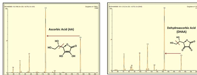
Figure 1. Fragmentation patterns of AA and DHA, showing fragment ions used for negative ion ESI-MS/MS analysis.
